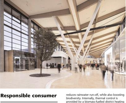
Located north of Vienna, ATP Architects' G3 Shopping Resort Gerasdorf features one of the largest timber roofs in Europe. Supported on pairs of Y-shaped steel columns, the 20,000 square metre undulating roof structure is constructed from glulam beams, laminated engineered timber panels and plywood. The carbon dioxide held within the timber equates to a saving of around 23,000 tons. Over 3000 square metres of sedum roofing
