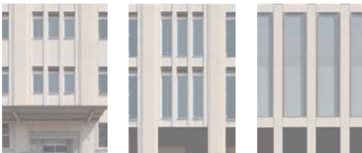
Façade concept: from left: existing, refurbishment, addition
